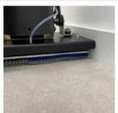
**Edge-to-edge Cleaning** unlike circular rotary machines, The Ocelot's rectangular drive board allows edge-to-edge cleaning.
